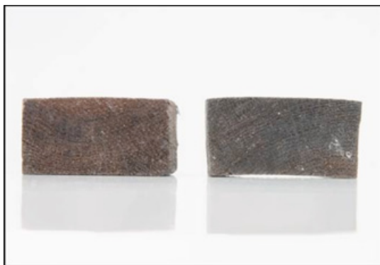
Photograph N°1: Shrinkage effect observed on samples not treated by PEG (left) compared to sample treated with 30% wt PEG 4000 (right).
