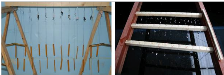
FIGURE 2: Hanging construction of the samples in two different depths (left) and installation in the storage basin (right).
